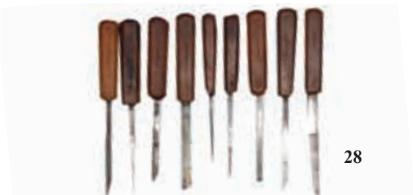
28. A fantastic set of nine plane makers floats, found in Glasgow and the gentleman's father worked at the MATHIESON factory, G++ (200-300)
