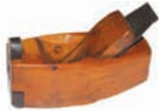
16. A solid boxwood compass plane with adjustable nose, G+/G++ (30-50)
