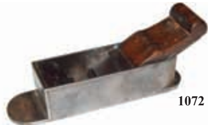
1072. An early 8" dovetailed mitre plane (150-250)
