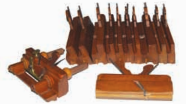
14. An extremely superb set of wooden planes. A full set of even hollows and rounds, ten graduated side beads, a twin iron tongue and groove plane and a lovely screw stem sash fillister all by COCKBAIN, Carlisle, same owner W. Backhouse, MINT CONDITION, RARE, F (900-1200)
