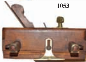
1053. An elusive sash fillister by OSBORN with the extra brass fence for "off the bench" work and "on the bench work" with boxwood fence (60-90)
