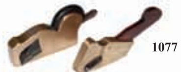
1077. Two small brass rebate planes, one is compassed (70-100)
