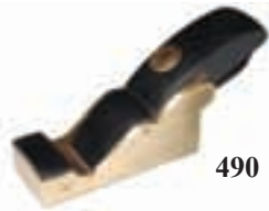
490. A very high quality brass chariot, steel soled, blade is marked "PENTONVILLE STREET" 4 1/4", ebony infill (100-150)
