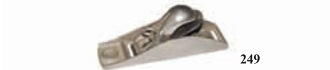
249. An unusual nickel plated reversible block plane (30-50)
