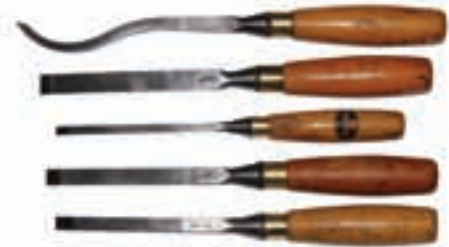
173. Four graduated mortise chisels and a lock mortise chisel, all boxwood handles, all by MARPLES , G++ (80-120)
