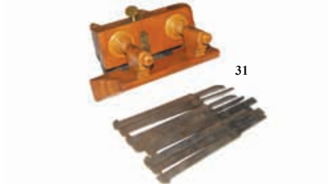
31. A lovely screwstem plough by PRESTON with a set of original PRESTON irons, wrong wedge, otherwise G++/F (100-150)
