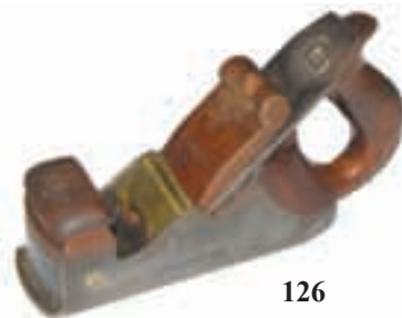
126. A very elegant 7 1/2", early, iron, Scottish smoothing plane with lovely cupid's bow brass bridge, G++ (120-180)
