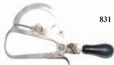
831. An unusual calibrated calliper with ebony handle, marked "INDICATING CALIPER COMPANT NEW YORK, PATENT AUG 8 1916 FEB 25 1919" (50-100)
