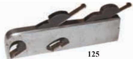
125. A twin iron dovetailed rebate plane marked SPIERS AYR on the metal, G+/G++ (120-180)
