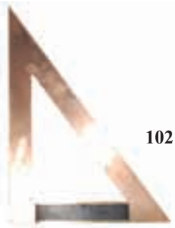
102. A quality level combined with brass trisquare, F (50-80)
