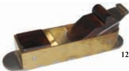
121. A 10 3/4" dovetailed brass mitre plane, steel sole, rosewood infill, G+/G++ (200-300)
