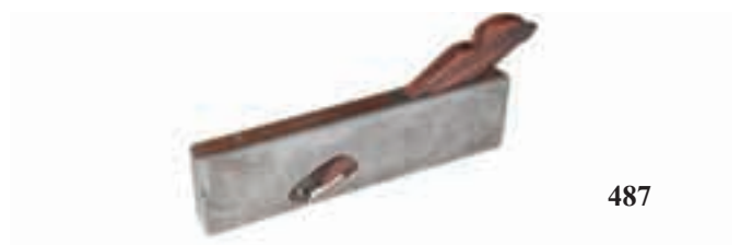
487. A dovetailed steel rebate, 8 3/4" x 5/8" (70-100)
