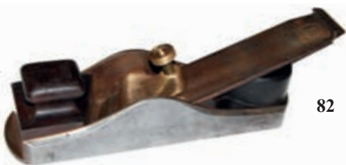
82. A NORRIS jewel. A 10 1/2" No.11 mitre plane with skew mouth. Blade by IBBOTSON not numbered but almost certainly original, slight superficial pitting but no other faults, RARE G+/G++ (1500-2500)
