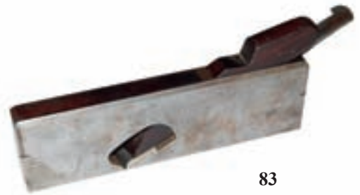
83. A 9" x 1" skew mouthed rebate plane marked MELHUISH but almost certainly made by NORRIS, a few spots of pitting otherwise G+/G++ RARE (100-150)
