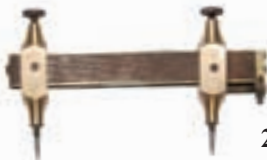
26. A most unusual pair of 2 1/2" brass trammels with an adjusting mechanism, G++ (70-100)
