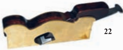
22. A NORRIS No.20 gunmetal shoulder plane, steel soled, 1 1/2" wide, NORRIS blade, G++/F (250-350)
