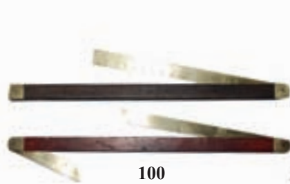
100. Two boat builders bevels, one has the unusual feature of a calibrated arm and stock, G++ (60-90)
