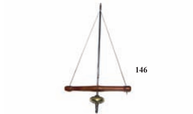
146. A pump drill with solid brass weight, 16" tall, G++ (40-70)
