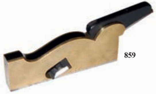
859. A good quality steel soled rebate plane, 5 3/4" by 11/16" (60-90) 860. Three good bowsaws (30-50)
