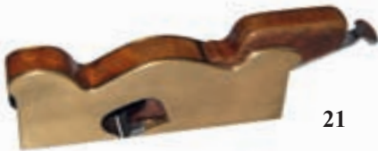
21. A NORRIS No.20 gunmetal shoulder plane, steel soled, rosewood infill, 1 1/4" wide, NORRIS blade, G++ (200-300)
