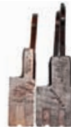
180. A RARE twin iron cocked bead by MALLOCH and a single iron by MOIR, both 7 1/2" long, G++ (30-50)
