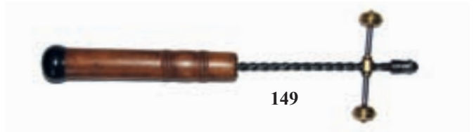
149. A most unusual Archimedes drill with bits contained in the handle, 14 1/2", G+ (40-70)
