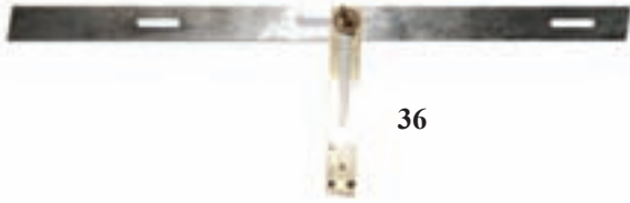
36. A most unusual brass and steel 24" adjustable sliding bevel. It has the facility to move the stock into three positions on the arm marked "PAT APL'D FOR MAY 2, 1889" G+/G++ (100-150)
