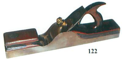
122. A 17" iron infill jackplane, attractive construction, G+/G++ (120-160)
