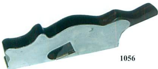
1056. An 8" x 1 1/4" dovetailed shoulder plane (70-100)
