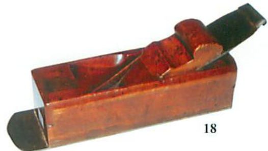
18. A 10" wooden mitre plane with steel sole and sneaked iron, G++ (70-100)
