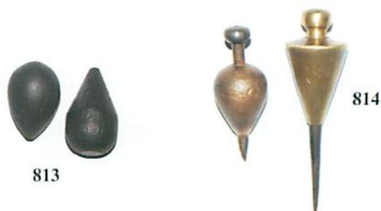
814. Two early 19th Century plumb bobs (both steel tipped), a 4" bronze and iron and a 6" brass and iron (80-120)
