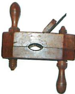
1031. An impressive wheelwrights rounder by VARVILL (70-100)
