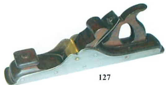
127. An extremely stylish 17 1/2" iron jackplane, lovely shape to metal body, G++ (150-250)
