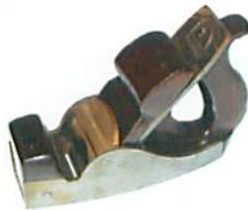
118. An attractive iron infill smoother with early style brass bridge, 7 3/4". Quality rosewood infill and wedge, G++ (100-150)
