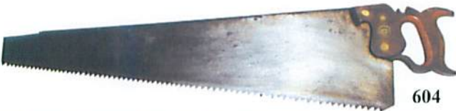
604. An early rip saw 3tpi with the established 1770 brass button, G+/G++ (40-70)
