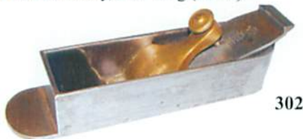
302. A dovetailed SPIERS mitre plane 10 ½" long, original snecked iron (short) G++ (300-500)
