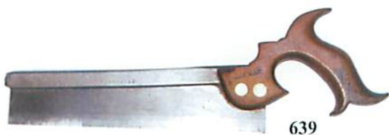
639. A scarce 10" steel back tenon saw by FITCHEW , G+/G++ (30-50)
