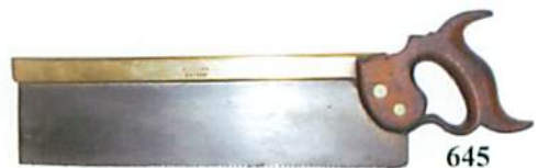
645. A 14" brass back tenon saw by HOLLAND , London (30-50)
