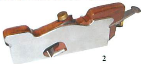
2. A NORRIS A7, adjustable shoulder plane, slight pitting to the top of the blade otherwise G++ (1000-2000)
