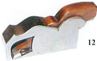
12. A NORRIS No.25 malleable bullnose, replaced blade, G+/G++ (100-200)
