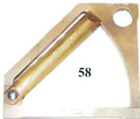
57. A most unusual levelling device marked "A WORKING LEVEL OF WATER" and "SHIPSTON ON STOUR", G++ (80-120)
