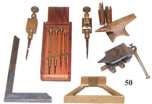
50. Two small anvils, a pair of brass trammels, a mitre template, early steel square and a brass combination tool (40-70)
